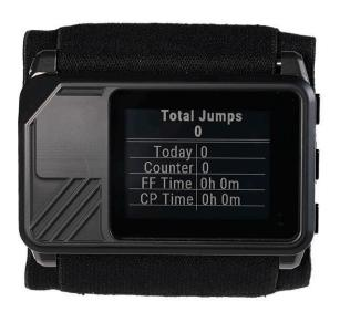
This screen gives an overall view of jump numbers, how many jumps have been performed today, and total accumulated times for freefall and canopy.
