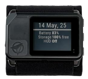
The info screen displays the date at the top of the screen. The remainder of the screen is split into sections:
