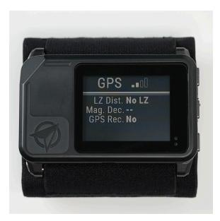
The GPS screen displays information related to the GPS capabilities of the Stratos. The rows from top to bottom on this screen are:
