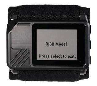
Selecting this menu item will restart the device in USB mode. Connect the device to a computer or smartphone after it has restarted to view it as a USB storage device. The jump log will be accessible as a comma separated value file (logbook.csv).
