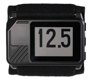
The altitude screen will automatically display whenever the Stratos is descending fast enough to be considered freefall speeds. There is no way to change the screen while the altitude is being displayed, and all buttons are disabled.
