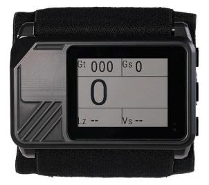
The ascent screen will display automatically when you take off in an aircraft and begin to ascend. If you are in a menu this won't happen automatically. You can exit the menu and use the up/down buttons to scroll through screens in order to find the ascent screen.
