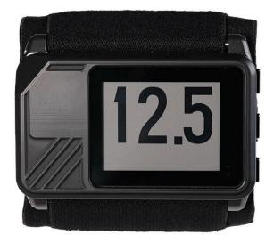
The altitude screen will automatically display whenever the Insight is descending fast enough to be considered freefall speeds. There is no way to change the screen while the altitude is being displayed, and all buttons are disabled. The altitude will be shown in one of these 3 formats (depending on the altitude and descent rate):
